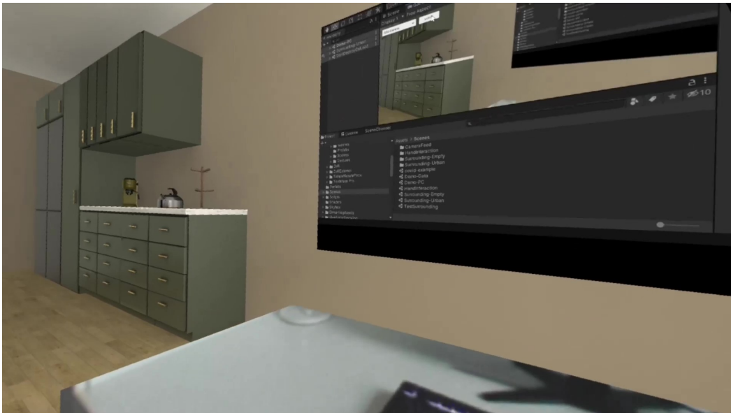
Figure 5.1: In this demo, the object reference's shape is a cube which frames a physical desk. Additionally, a computer screen is streamed into the virtual environment. This application allows the user to develop and adjust a virtual reality application directly in Unity without removing the headset.
